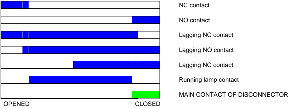
Figure 4 Pilot switch, functional diagram
